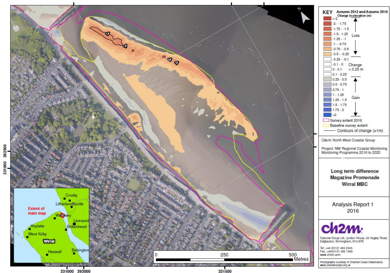
Figure 17: A topographic difference map for the frontage between Tower Groyne and Egremont Groyne which shows the difference in beach levels between Autumn 2012 and Autumn 2016. Red is erosion and blue is accretion.
