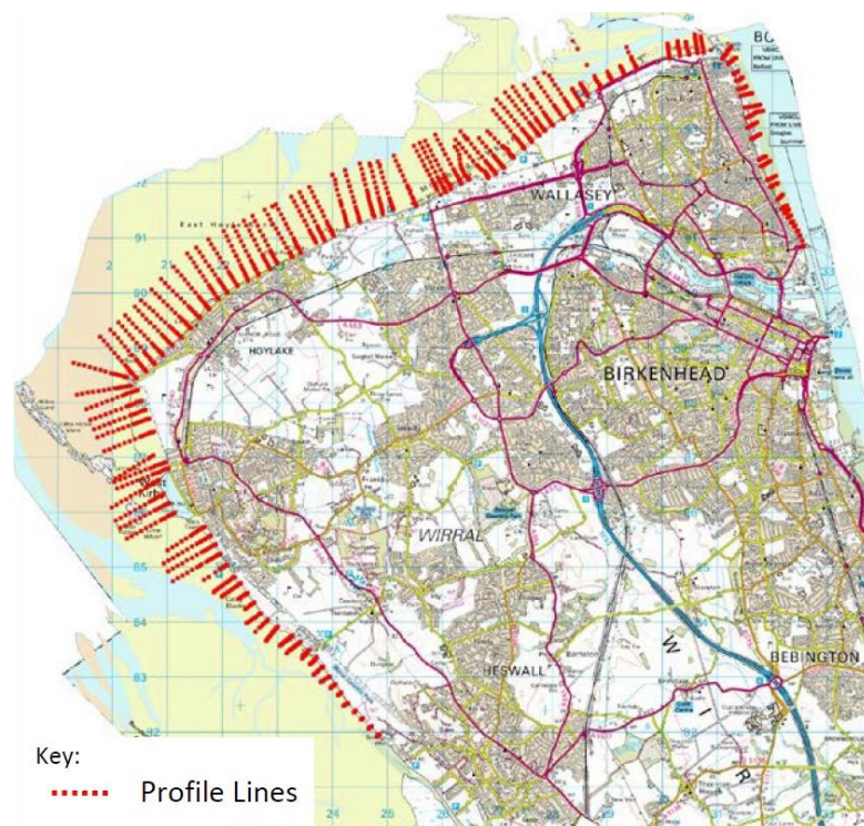
Figure 7: The location of the 133 beach profile lines along the Wirral coast. Image source: Sefton Council (2016) Background mapping provided by Ordnance Survey © Crown Copyright and database rights 2014 Ordnance Survey 100018192.
